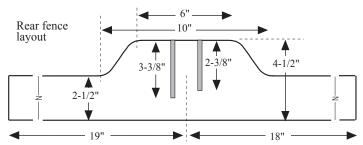
Note: center offset and groove positions must be reversed in front fence.
